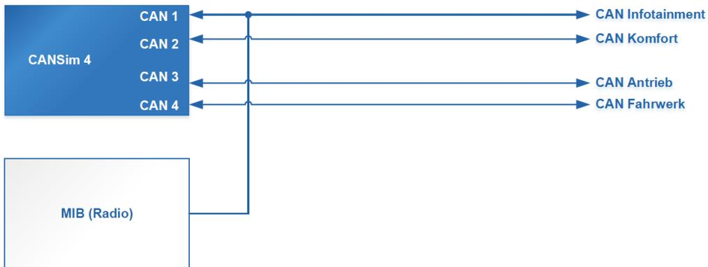
Figure 8: Connection Diagram of Modes 2 and 3 without Gateway
