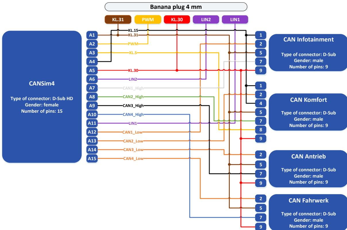
Figure 20: Full Octopus Cable Harness – Schematics
