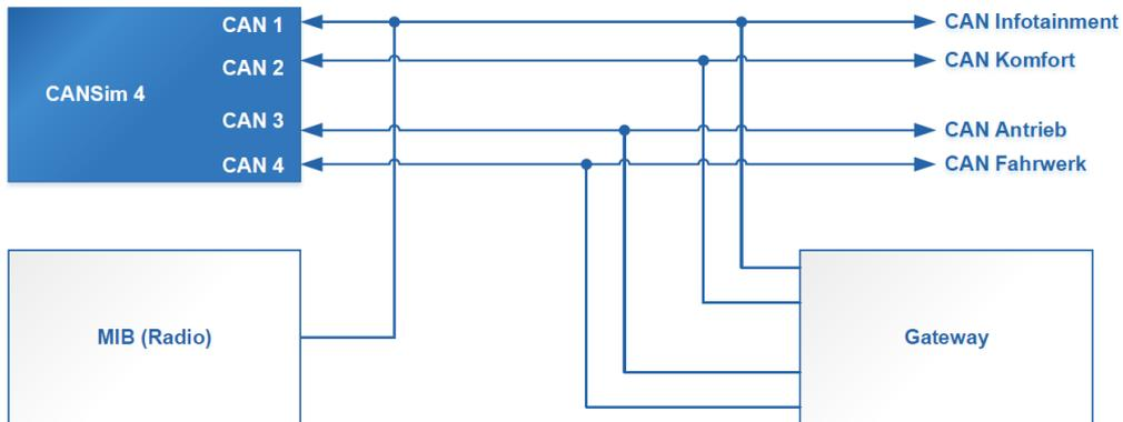
Figure 7: Connection Diagram of Modes 2 and 3 with Gateway and Radio
