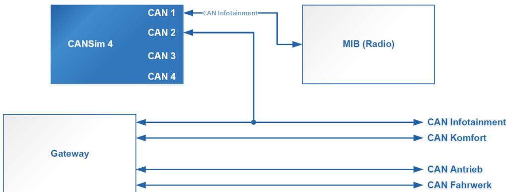
Figure 5: Connection Diagram of Infotainment Gateway Mode MQB / MQB37W
