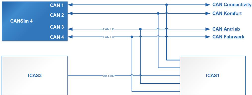
Figure 11: Connection Diagram of MEB Mode 6
