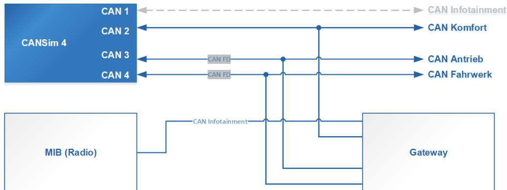
Figure 10: Connection Diagram of MQB / MQB37W Mode 4
