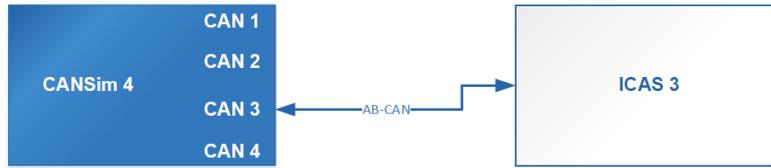
Figure 6: Connection Diagram of Infotainment Simulator Mode MEB
