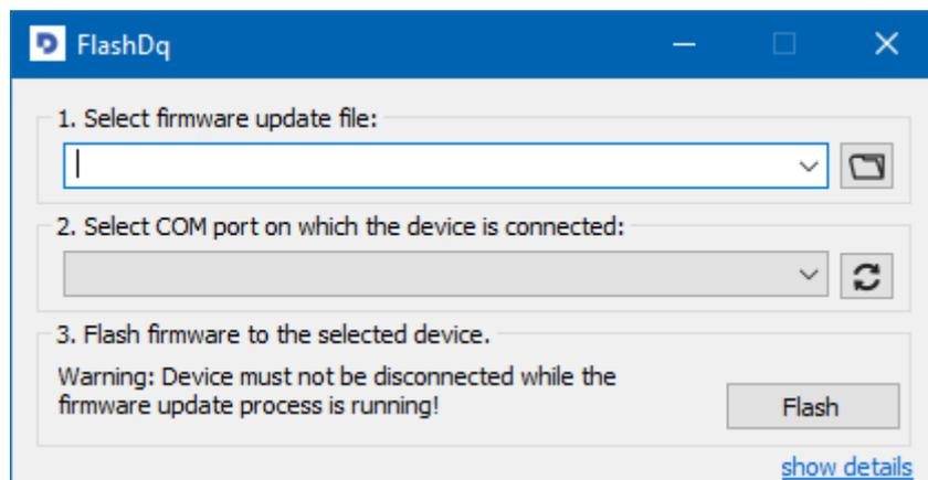
Figure 13: FlashDq Application GUI
