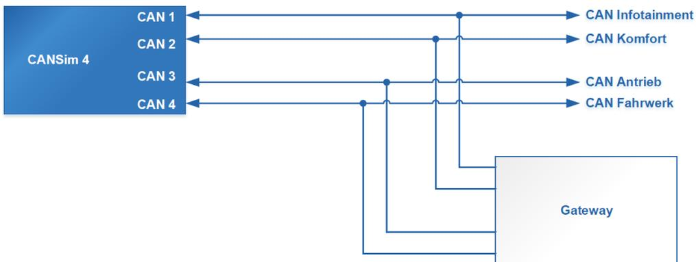
Figure 9: Connection diagram of Mode 2 and 3 with gateway and without radio
