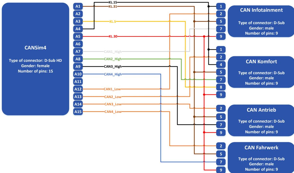
Figure 18: Octopus Cable Harness – Schematics
