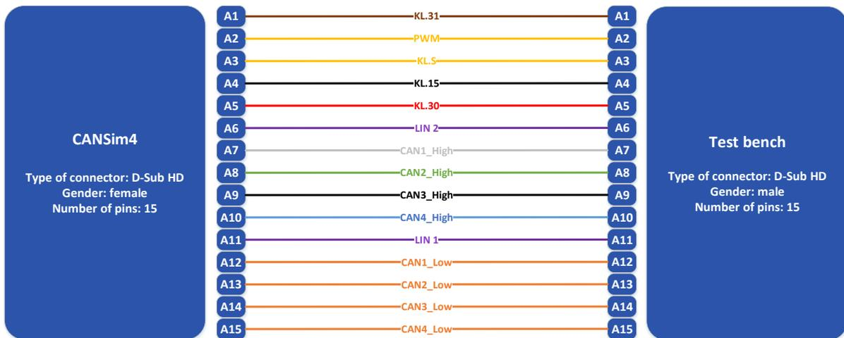
Figure 16: Cable Harness 1:1 – Schematics
