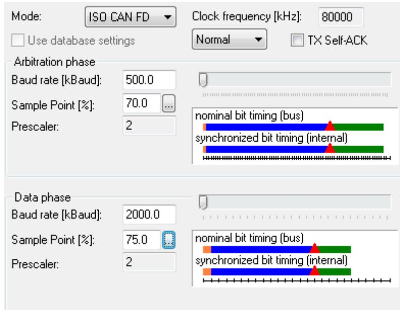
Figure 2: CANoe CAN FD Settings Dialog Matched with CANSim Test Mode
