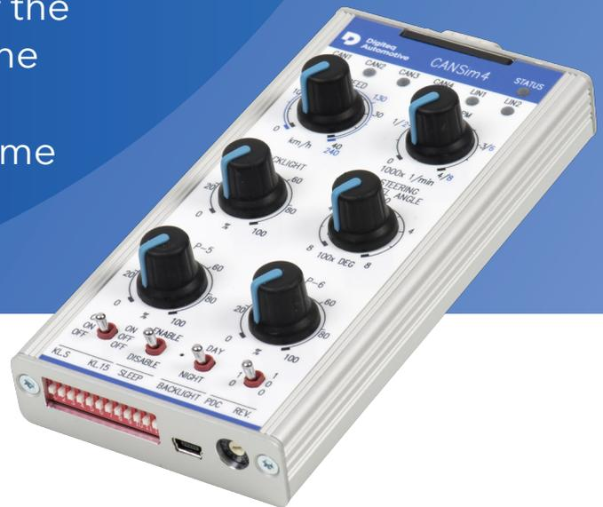
It is mainly used for testing MIB and ICAS units. It can also be used for testing other units, in various demonstrators and in all use-cases, which require CAN simulations.
